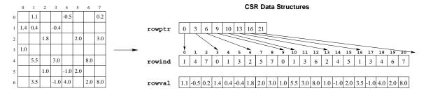
Figure 17: An example of the CSR format for storing sparse matrices.
